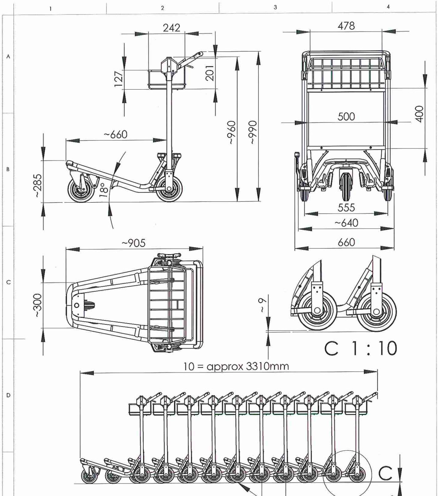
\* due to the nesting procedure the height of the nested row is slightly inclining maximum height is reached approx. with the 12th trolley
